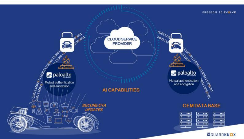
Palo Alto Networks<sup>®</sup> GlobalProtect<sup>™</sup> Cloud Service secures the external network between the vehicle and the OEM cloud through the use of their secured communication channel while GuardKnox provides a holistic lockdown approach to the vehicle's internal network by enforcing strict set of rules on all incoming and outgoing communication in real time.
